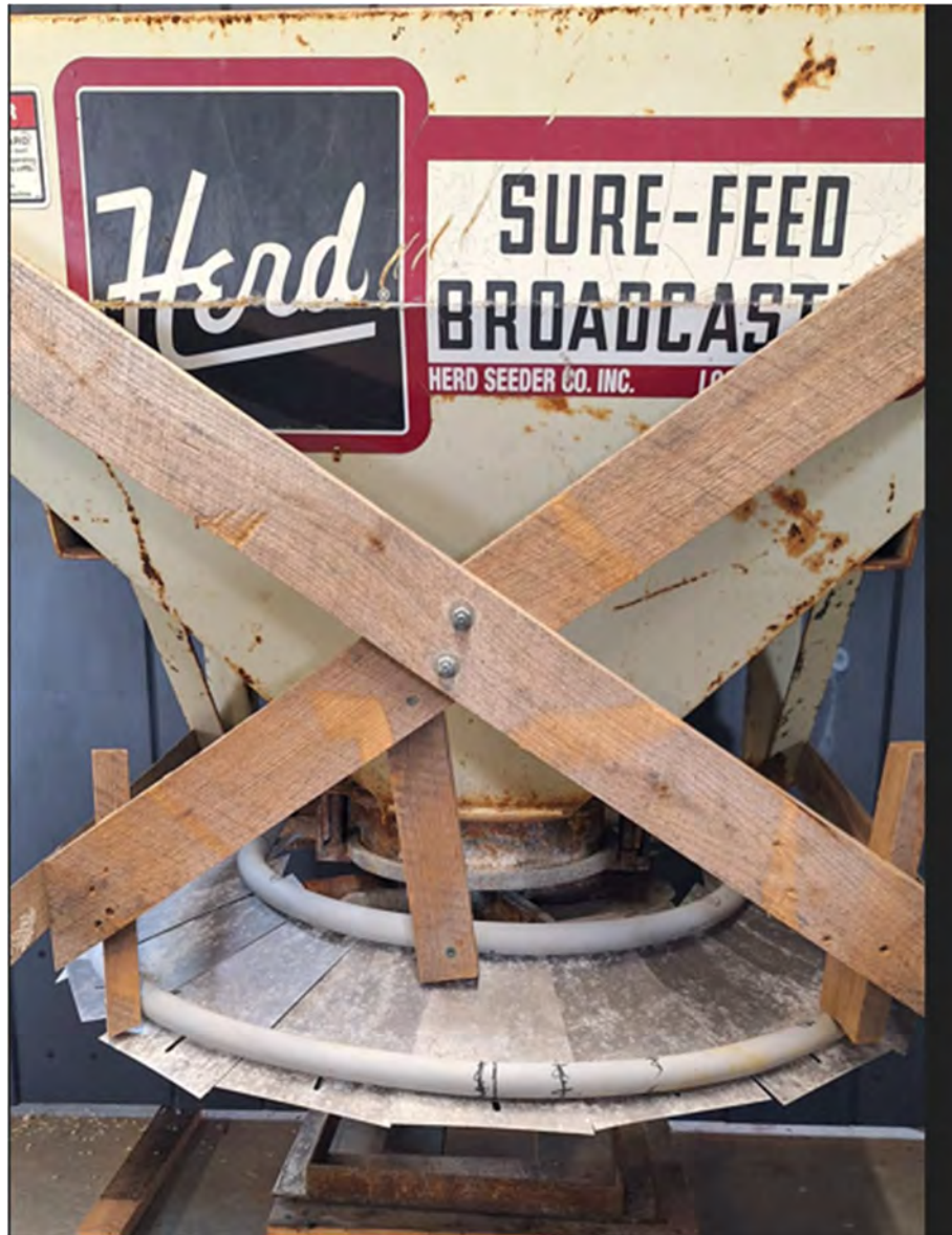
3pt hitch Herd broadcast spreader with a custom fully adjustable shroud used to spread at the desired 6 foot width
