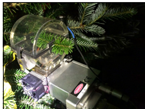
Above: Dendrometer bands are used to measure tree trunk growth. Below: A conifer chamber is used to measure a Fraser fir's photosynthesis, the process by which a tree makes sugars, and transpiration, which is the tree's water loss.
