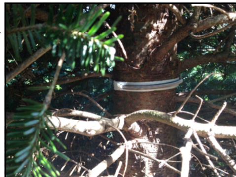
Above: Dendrometer bands are used to measure tree trunk growth. Below: A conifer chamber is used to measure a Fraser fir's photosynthesis, the process by which a tree makes sugars, and transpiration, which is the tree's water loss.
